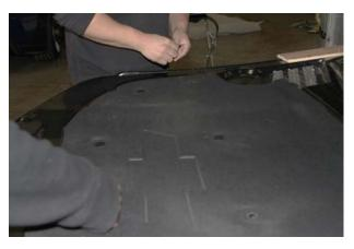
**Step 10:** If you want to install windshield washer nozzle, carefully remove the windshield washer hose from the OEM hood by unclipping it. You may have to twist and wiggle it around. Be sure to also remove the plastic frame that is attached to the hose (if applicable).
