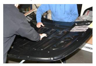
**Step 9:** Place the OEM heat shield on the carbon hood and proceed to reinstall the heat shield clips taken off in Step 4. \*It may be necessary to enlarge the holes on the hood's skeleton. These are purposefully smaller than OEM to ensure a snug fit.\*
