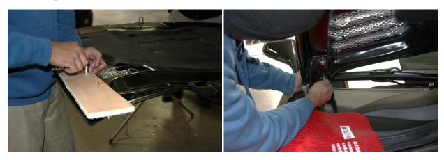
**Step 4:** Look at the underside of the hood. At this point you want to determine whether you can transfer your OEM heat shield onto your carbon fiber hood. The hood's style will determine if a heat shield transfer is possible. **If you cannot transfer the heat shield, proceed to step 10.** Be advised that you can purchase an aftermarket heat shield online. The use of a heat shield will help protect your carbon hood from damaged caused by engine heat.
