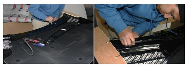
**Step 12:** In some cases, depending on the vehicle you have, you may have to/want to transfer your OEM striker onto your new carbon fiber hood. To do this, simply unbolt the striker and screw it onto the carbon hood.
