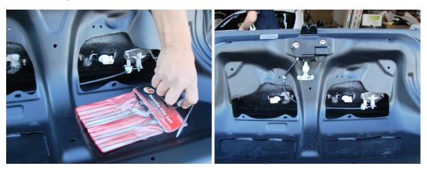
**Step 10:** If applicable, reinstall tail garnish by carefully pushing the garnish into the trunk. Be sure to screw garnish on securely.
