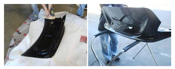
**Step 6:** With the help of a partner, perform a quick installation to visually inspect how the trunk will fit on the car. Attach the hinges, and carefully close the trunk. Make sure that the overall body lines are smooth.
