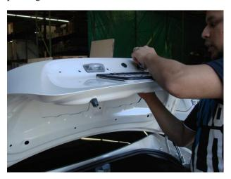
**Step 3:** Remove the trunk's shocks. In our case we inserted a flathead screwdriver between the hinge and shock and then carefully pulled the clip and shock simultaneously.
