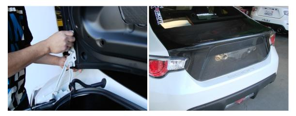
**Step 7:** Carefully remove the trunk. If applicable, install license plate lights onto the carbon trunk. (Note: light holes are intentionally made smaller than OEM to ensure a snug fit. To resize, use a file.)
