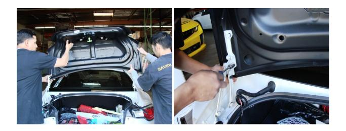
**Step 12:** With the Seibon Carbon trunk installed, reinstall the tail light harness. At this point, you can reinstall your trunk cover (if applicable).
