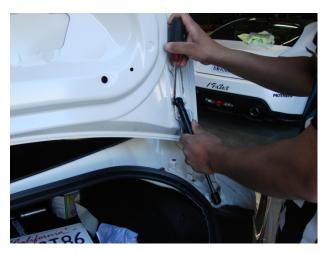
**Step 4:** Remove the OEM factory trunk by removing the bolts/nuts attaching it to the hinge. (Note: you may need a partner to help hold the trunk while you are unbolting the trunk.) Place the trunk where it will not get damaged.
