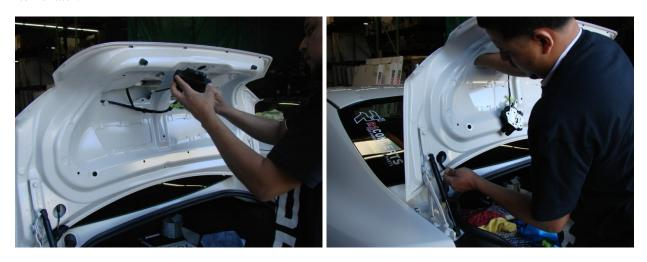
**Step 2:** If applicable, remove the trunk's tail garnish by pulling it. Proceed to carefully remove license plate lights.
